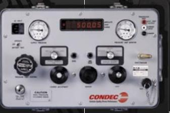
cylinder built in, and uses nitrogen to eliminate the mess and leaking of hydraulics. As the tests required are dead-ended and usually performed on a small diaphragm device, the CONDEC performed many tests from the easily rechargeable cylinder – even at pressures to 2000 psi.
